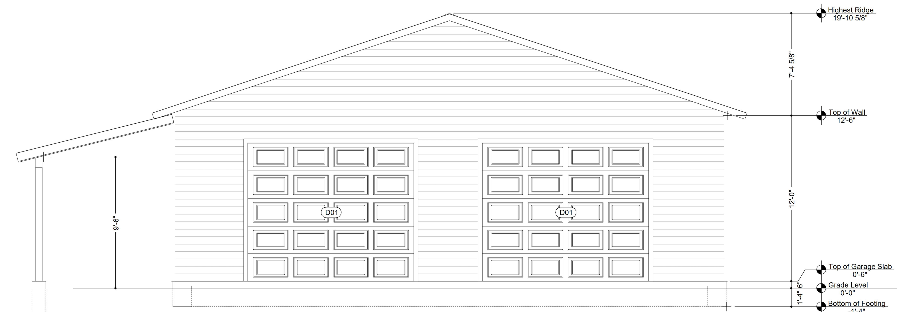
FRONT ELEVATION SCALE: 3/16" = 1'-0"
